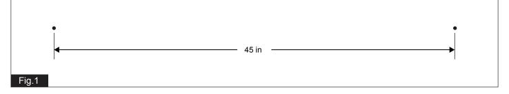
1. Select suitable location that can support the weight of the fixture and has an outlet on the ceiling to insure that the fixture hangs properly.Determine method of mounting before drilling.Make two spots on the ceiling 45 in. apart for the two anchors.
