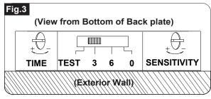
the knob counterclockwise. The delay may be adjusted from a minimum of 5 seconds to a maximum of 3 minutes. The light will stay on as long as motion is detected continuously and will automatically turn to low-level brightness when no more motion is detected after the delay time has passed.
